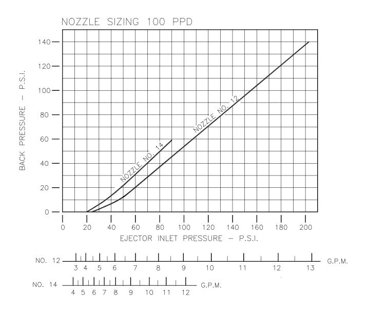
**NOTE:** For high altitude operation when using the ejector with the 480 and 200 Series vacuum regulators, with a supply pressure of 150 PSIG or less, increase the supply pressure by 1.0 PSIG for each 1000 feet above sea level for proper operation.
