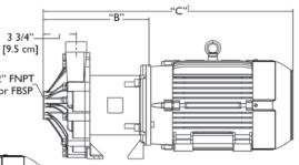
Also available 2" x 2" or 3" x 2" 150 lb. ANSI/ISO PN20/PN40/JIS 10K or 63mm x 63mm union connection. Flanges are in compliance with bolting dimensions only.
