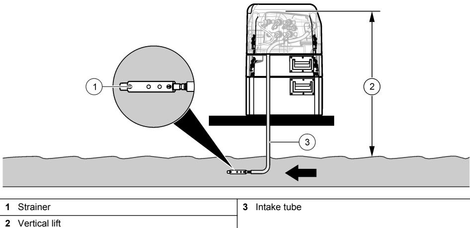
**Figure 8 Intake tube installation**
