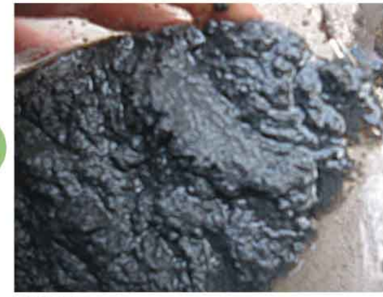
濃縮後 Sludge Thickening
