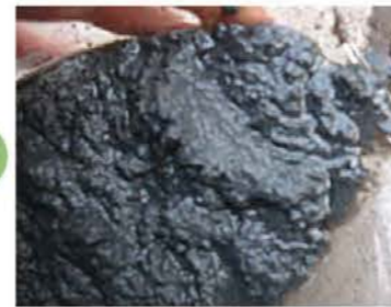
濃縮後 Sludge Thickening
